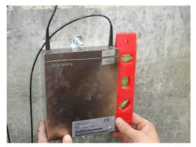
Fig. 2.6 Vertical alignment using a bubble level
