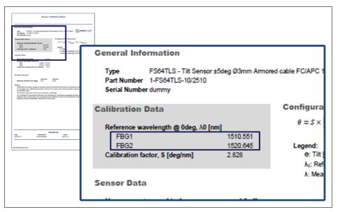
Fig. 2.11 Calibration sheet example - FBG wavelengths
