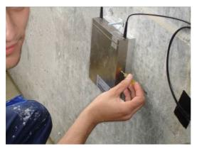
Fig. 2.10 Side locking screws (number "3")
