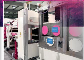
Longitudinal slitting shears - thickness profile
