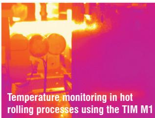
Temperature monitoring in hot rolling processes using the TIM M1
