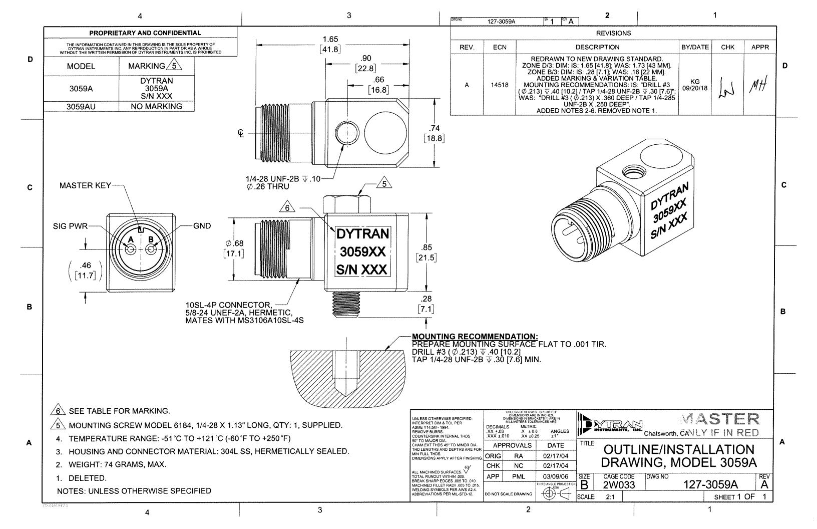
Model Number DOC NO PERFORMANCE SPECIFICATIONS PS3059A 3059A IEPE ACCELEROMETER REV C, ECN 15841, 07/13/20
