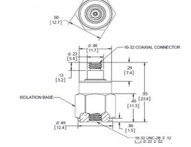
Units on the line drawing are in inches, units in brackets are in millimeters. Refer to 127-3056D9T for more information.
