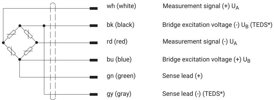
Cable shield, connected to housing
