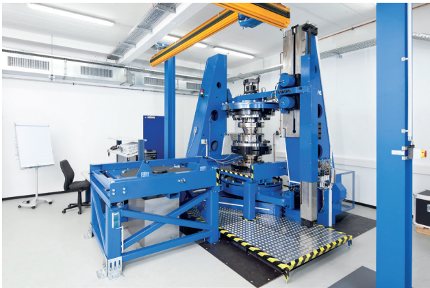
Top-quality test benches of HBM's own calibration laboratory ensure reliable measurement results of the T40.
