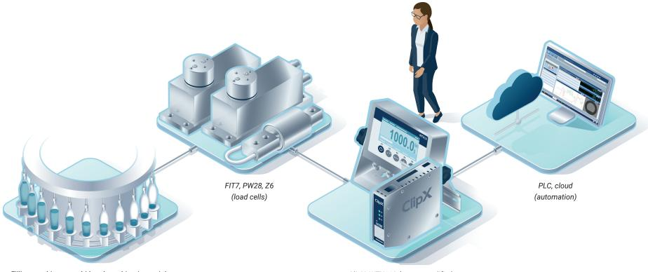
Filling machine or multi-head combination weigher
