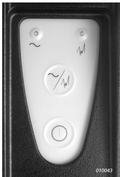
Fig. 2.6 Type 4297 control panel showing the start, sine wave/broadband noise selector buttons and LED indicators
