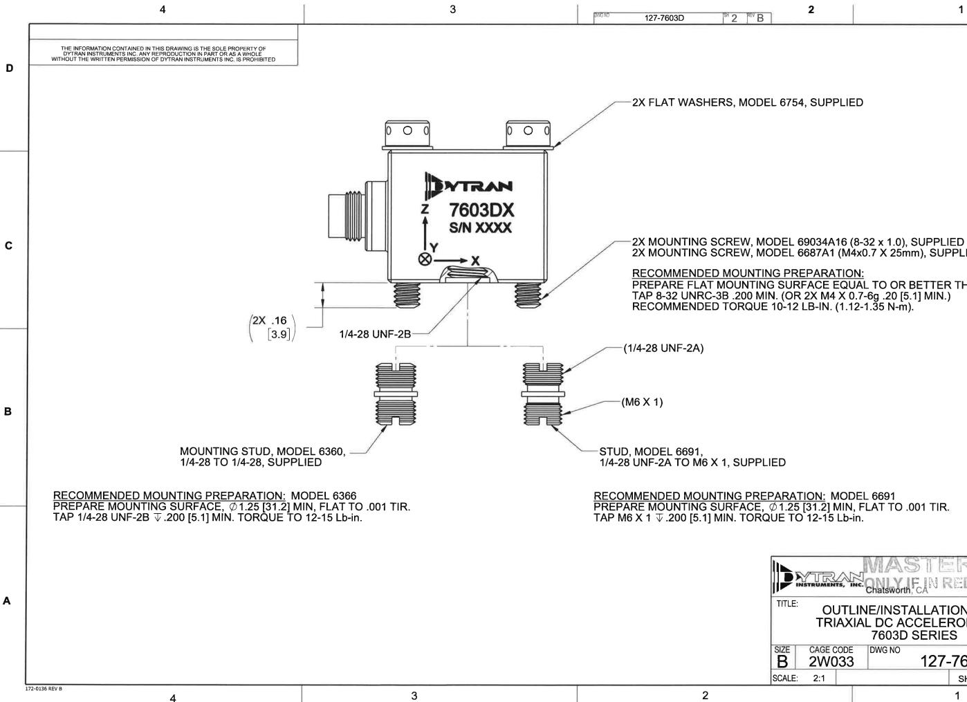
1 2 D С 2X MOUNTING SCREW, MODEL 6687A1 (M4x0.7 X 25mm), SUPPLIED PREPARE FLAT MOUNTING SURFACE EQUAL TO OR BETTER THAN.001 TIR. В INSTRUMENTS, INC. Chatsworth, CA Α OUTLINE/INSTALLATION DWG, TRIAXIAL DC ACCELEROMETER, 7603D SERIES DWG NO REV CAGE CODE 127-7603D 2W033 2:1 SHEET 2 OF 2
