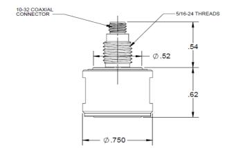
Units on the line drawing are in inches, units in brackets are in millimeters. Refer to 127-1050V for more information.
