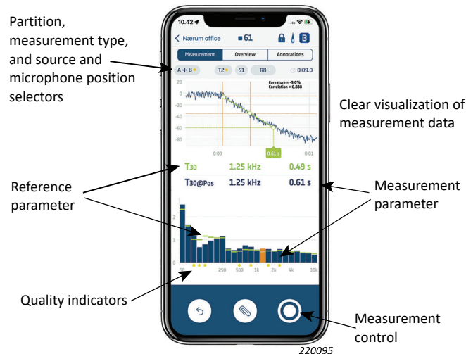
Fig. 1 The mobile app keeps you connected to your measurements
