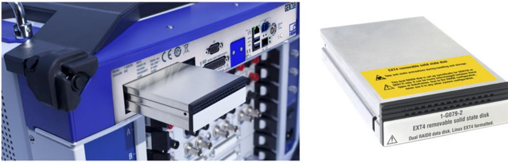
**Figure 1.18:** Example of SSD in drive carrier partially slid into GEN7tA (left) and SSD built inside drive carrier (right)
