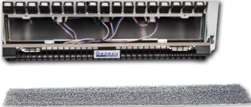
Figure 1.16: Easy access for cleaning/replacing air filter
