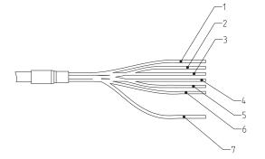
Contact 1 (white [WH]) = measurement signal (+) Contact 2 (red [RD]) = measurement signal (-) Contact 3 (black [BK]) = excitation voltage (-) Contact 4 (blue [BU]) = excitation voltage (+) Contact 5 (green [GN]) = sense line (+) Contact 6 (gray [GY]) = sense line (-) Contact 7 Shield (yellow [YE]) = Cable shield
